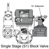
A2859-11 Block Valve and 3 Way Solenoid (PN 81527)
