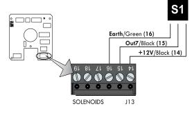
Solenoid 1 Wiring for Single Stage Valves
