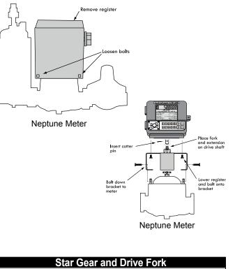
When the register is lowered onto a Neptune meter, make sure
