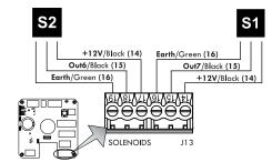
Solenoid 1 and Solenoid 2 Wiring for A2859-11 and 3-Way Two Stage, 2848-11 Two Stage, and E-7 Two Stage
